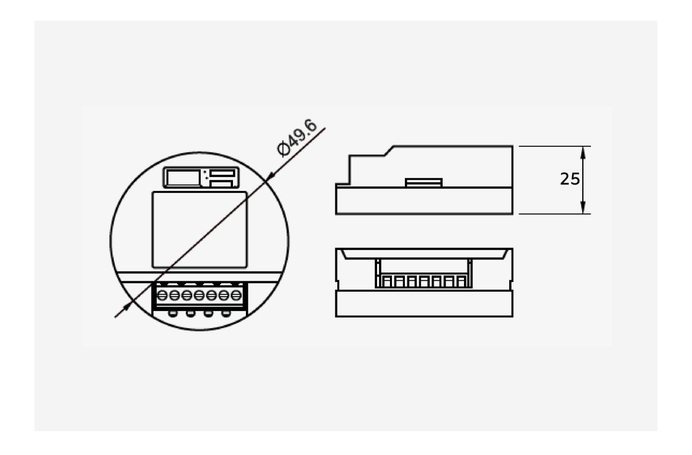
There are two connection options. The relay can be connected either as a power-free relay switch (NO) for garage doors and car gates or with supply power for door locks, magnets and strike plates.
