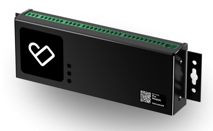
add up to two Wiegand based readers with PIN/RFID functions and there is a possibility to connect a door sensor and/or a motion sensor to trigger an alarm when there is any movement or an unauthorized entry at your site. Additional sensors can be applied via RS485.
